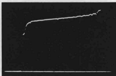
Fig. 7 -- Stress-time profile obtained for shock compression of \text{BaF}_2 in \langle 100 \rangle direction with an impact stress of 40 kbars.
